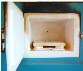
**Step 10.** Fire the piece face down at 1470° F (800° c) for 30 minutes. Remove from the kiln, allow to cool, and tumble with stainless steel shot for 30 minutes. Remove, dry, and prepare your work area for the resin inlay.
